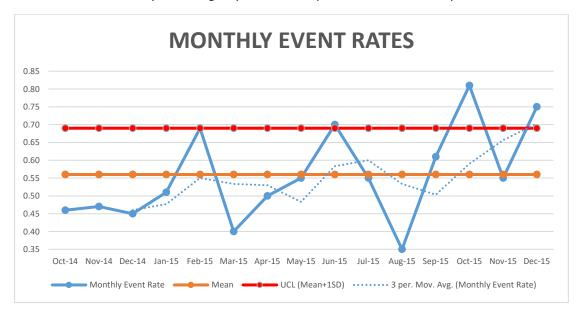
In connection with other standards like the Upper Control Limit (UCL)or the 3 month moving average, line diagrams provide an indication of performance of a specified system, and in the above case when and by how much the system has exceeded a particular control. The three month moving average can even be replaced with a linear or non-linear curve as a means of forecasting when an exceedance might occur.
