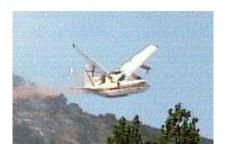
Lockheed C-130A Hercules registration N130HP, call sign Tanker 130, was flying against the Cannon Fire, near Walker, California on June 17, 2002, when it experienced structural failure of the center wing section, causing both wings to fold upward and separate from the aircraft. The fuselage rolled and crashed inverted, killing the three crewmen on board.
