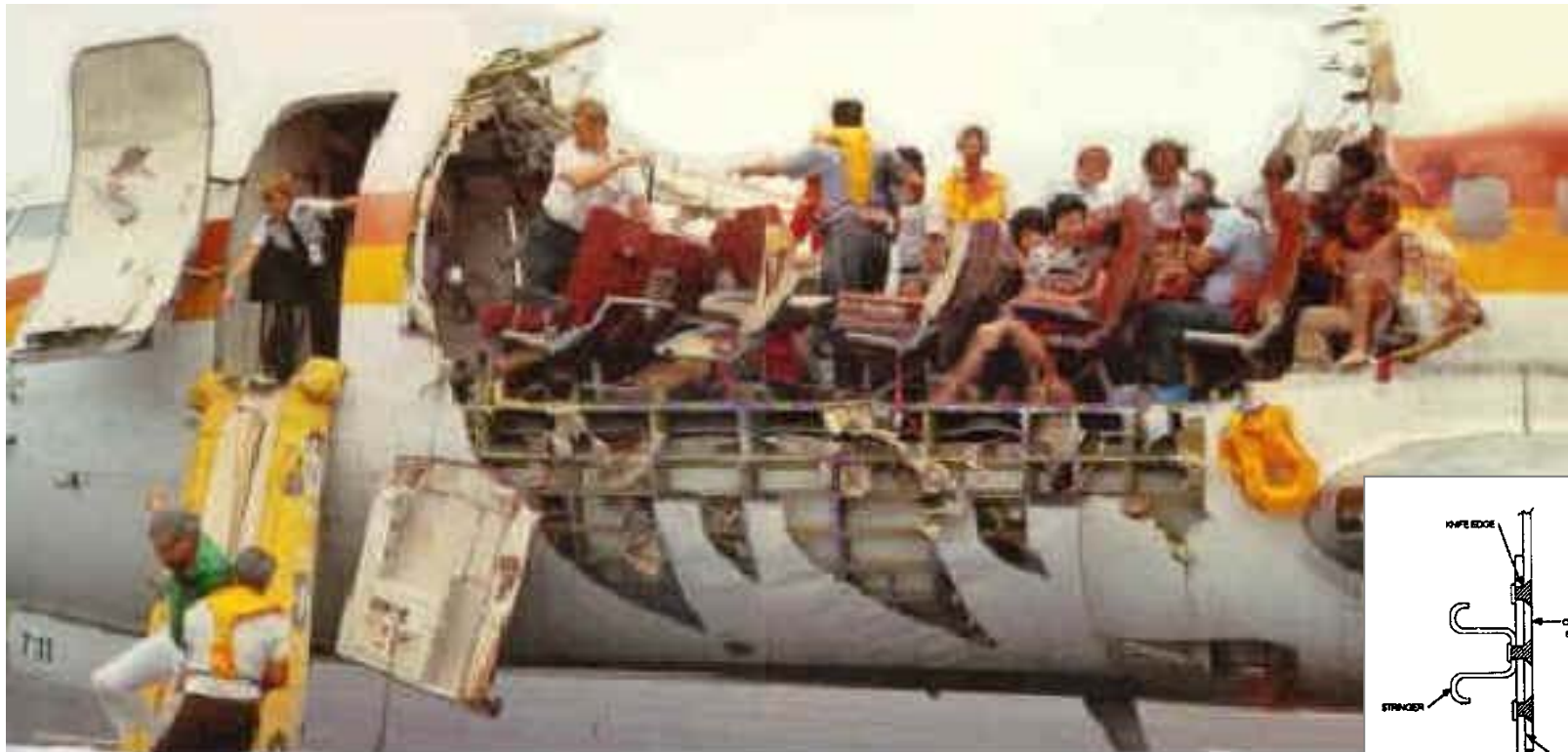
(missed cold bond lap joint disbond inspection SB 737-53A1039)
