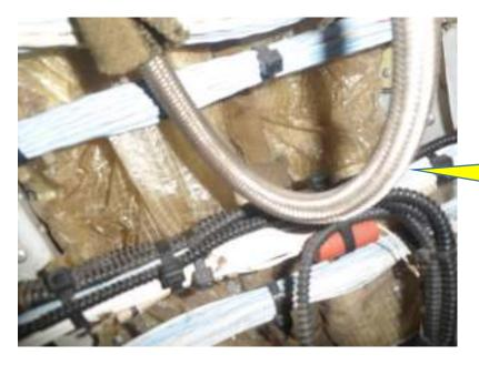
Captains oxygen pipe is in direct contact with wiring in several places!
