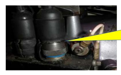
The integrity of sleeving designed to prevent the ingress of fluids and moisture into connectors must
