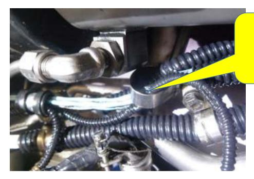
It is most important to ensure that all clips secure the cables effectively otherwise chafing can occur
