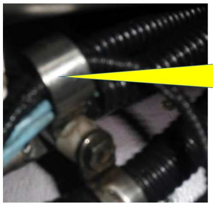
P Clips must be correct IAW IPC or other approved data and must afford appropriate support and protection, oversize P Clips pose a threat
