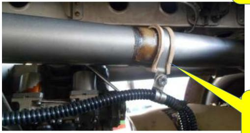
P Clip Migration all P Clips should be of the correct size and firmly attached e entire loom
