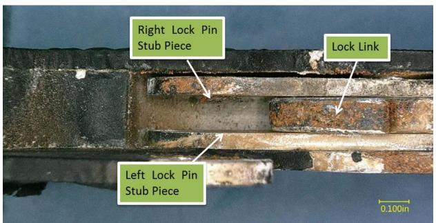
Figure 9a. Photograph of the left and right lock pin stub pieces.
