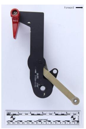
Figure 4a. Photograph of an exemplar gust lock handle in the ON position.
