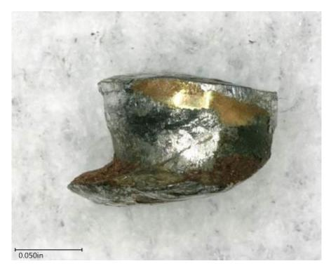
Figure 10. Photograph of the right lock pin stub piece.
