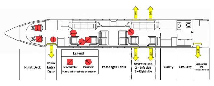
Figure 7. Diagram of the seating configuration showing occupant location and orientation.
