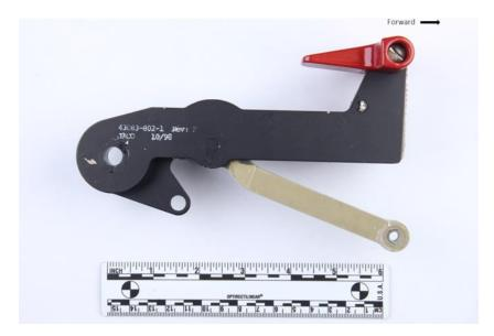
Figure 4b. Photograph of an exemplar gust lock handle in the OFF position.
