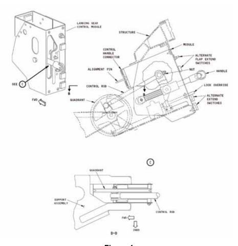
**Figure 1** Landing Gear Control Module showing handle and control rod
