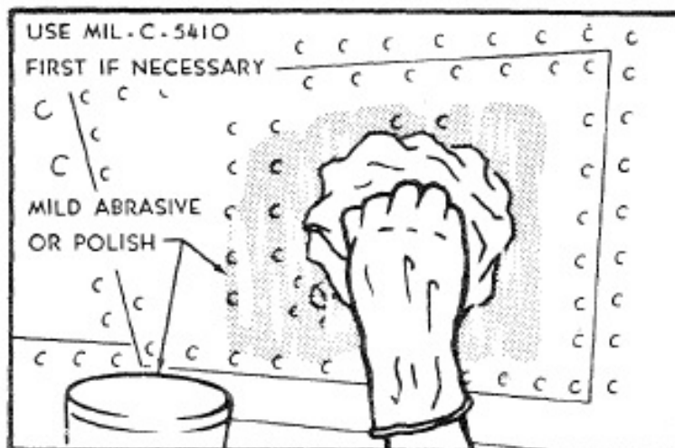
Figure 6-12. Polishing and Brightening Alclad Surfaces
