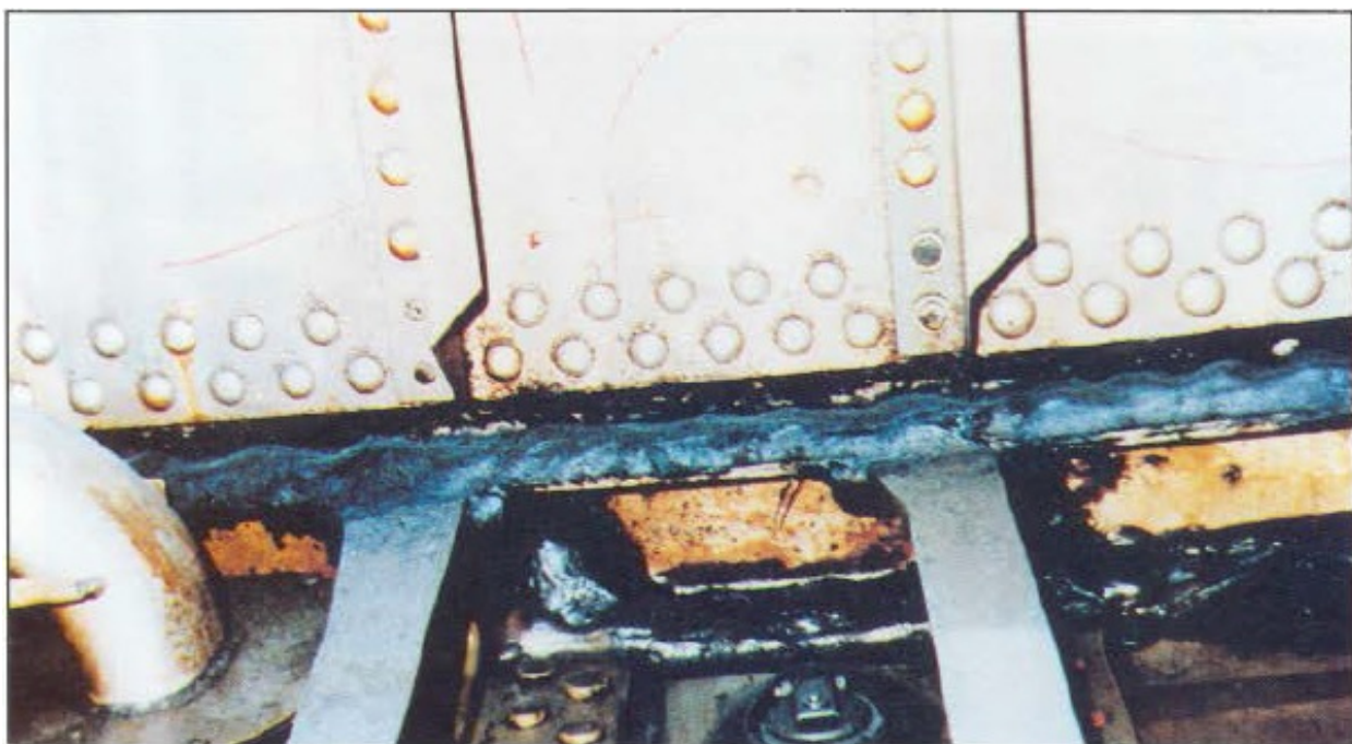
Figure 5-3. Corrosion Indicated by Blistering of Paint in Fuel Cell
