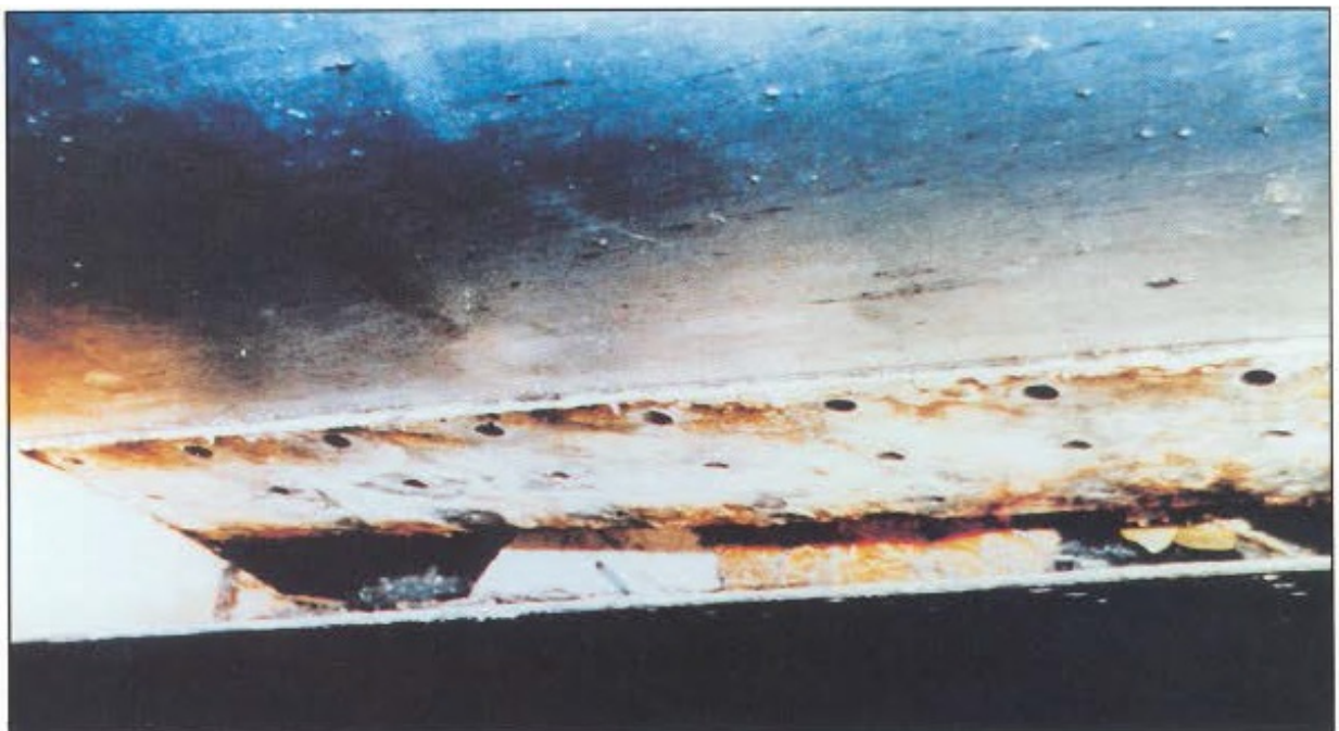
Figure 5-15. Severely Corroded Lap Joint
