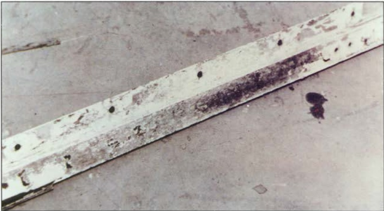
Figure 2-3. Uniform Etch Corrosion
