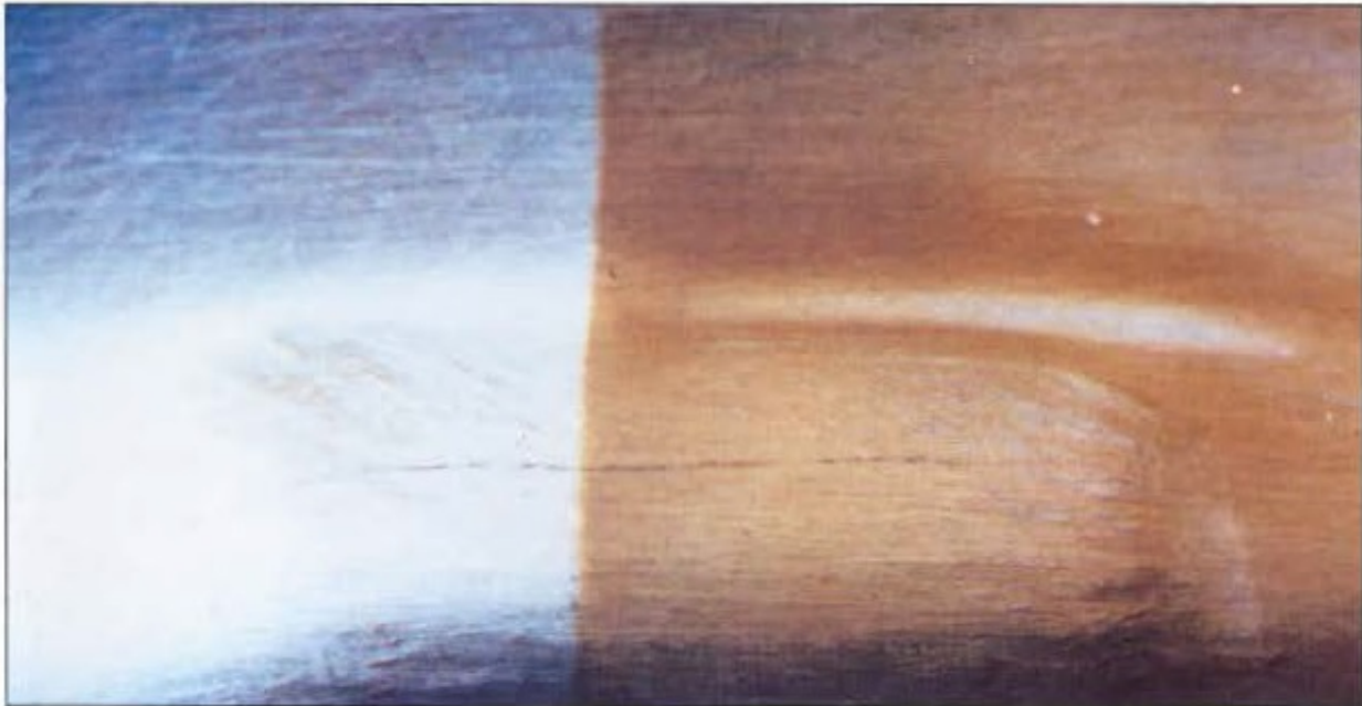
Figure 5-18. Bonderite 1200 Treatment Prior to Painting May Highlight Presence of Remaining Corrosion or Cracks
