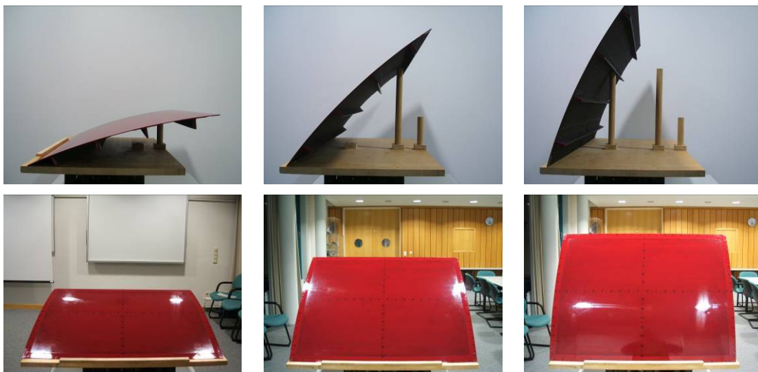
Figure 50: Inspection angles 15° (left), 45° (middle), 65° (right hand side)
