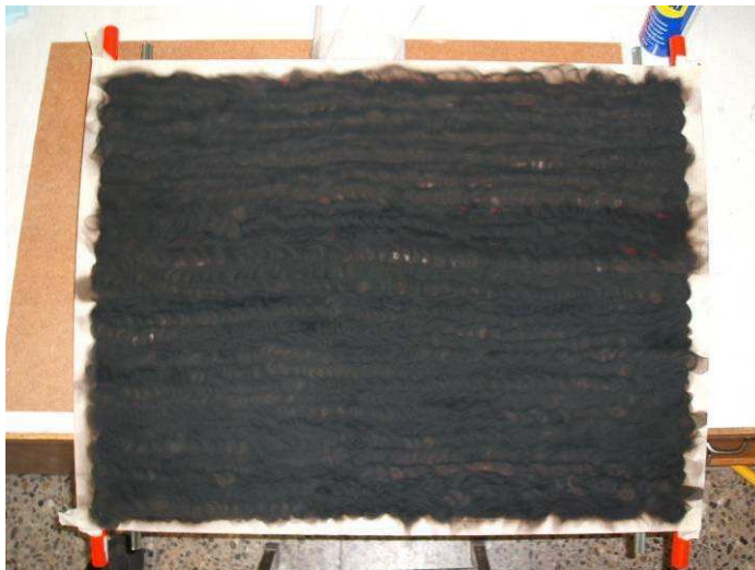
Figure 42: Panel 1 completely covered with soot from paraffin oil.
