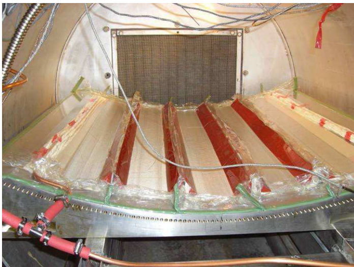
Figure 10: Stringers are supported by silicone cores (red pieces) with triangular cross sections to prevent them from collapsing during curing.
