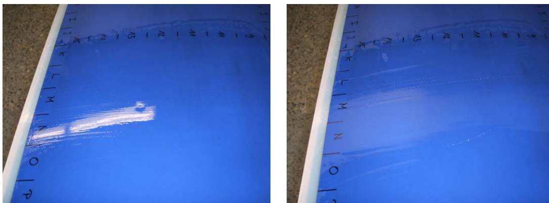
Figure 64: Surface wetting, to improve detectability of dents on matt surface.
