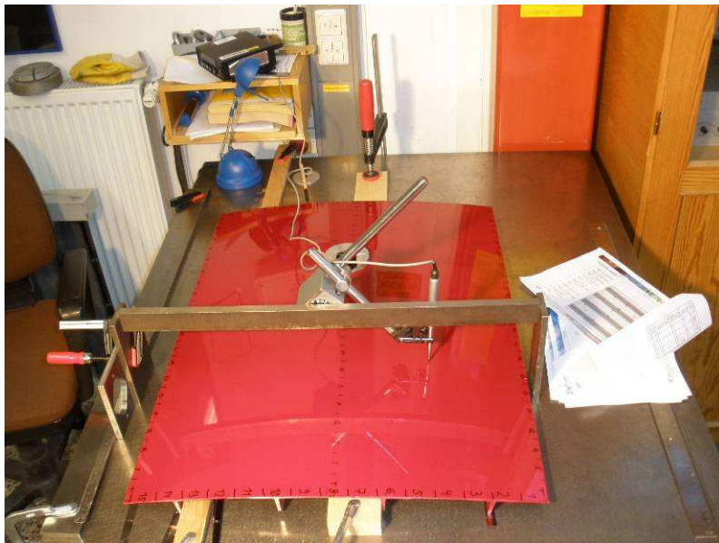
Figure 35: Set-up of dent depth measurements.
