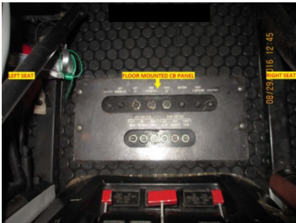
Figure 2 – Example of Floor Mounted CB Panel – Interior (1981 and later production)
